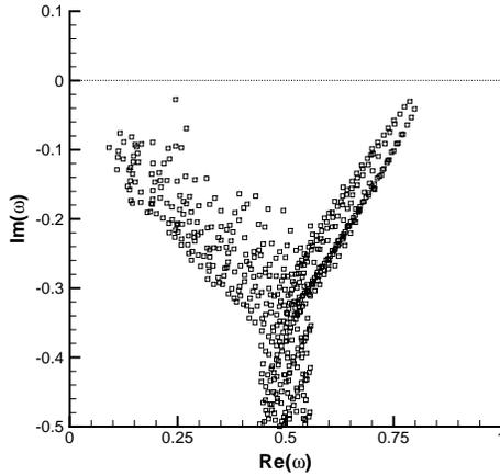
Figure 3. Discretized linear stability spectrum for aspect ratio  $A = 2$ , grid  $(65 \times 51)$ ,  $Re = 10400$  and  $\beta = 0.91$ .
