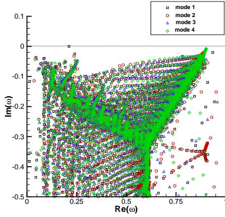
Figure 1. Complete spectrum of linear stability for a Poiseuille flow in a rectangular duct of aspect ratio  $A = 5$ . Grid  $(65 \times 51)$ ,  $Re = 10400$  and  $\beta = 0.91$ .
