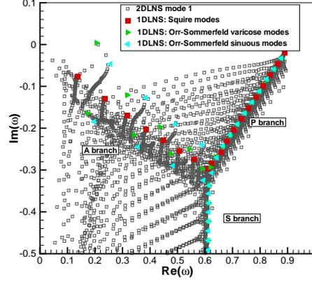
Figure 2. Poiseuille flow. Superposition of the linear stability spectra :  $\circ$  1D and  $\square$  2D (mode 1). Aspect ratio  $A = 5$ . Grid  $(65 \times 51)$  for 2D spectrum.  $Re = 10400$  and  $\beta = 0.91$ .
