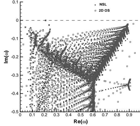
Figure 4. Poiseuille spectra (mode 1) obtained with different formulation of the equations of motion.  $\square$  : 2DOS;  $\circ$  : 2DLNS. Grids  $(65 \times 51)$ .  $A = 5$ ,  $Re = 10400$  and  $\beta = 0.91$ .
