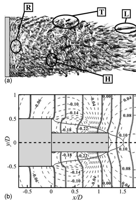
FIG. 4. (a) Snapshot of the coherent structures downstream of the step flow with their rotation visualized with an isosurface of  $QU_x^2/D^2=50$  colored by the sign of streamwise vorticity (white for positive and gray for negative). (b) time-averaged flow field. (—) Iso- $C_p$  with  $\Delta C_p=0.02$  between two lines, (—) isovelocity  $U/U_\infty=0.01$ , and (O) velocity profiles at several streamwise locations.
