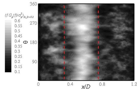
FIG. 6. (Color online) Spectral sheet of normalized premultiplied PSD of the pressure fluctuations at the wall  $fG_r(f)/\sigma_p^2$  for every streamwise and azimuthal locations along the emergence and for the particular dimensionless frequency  $St_D=0.2$ . (—) Spatial limits of the absolute area for  $m=1$ .
