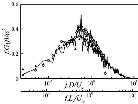
FIG. 5. Normalized premultiplied PSD of the pressure at the wall for the streamwise location  $x/D=0.99$ . (○) Ref. 17, (▲) Ref. 6, and (—) present calculation.
