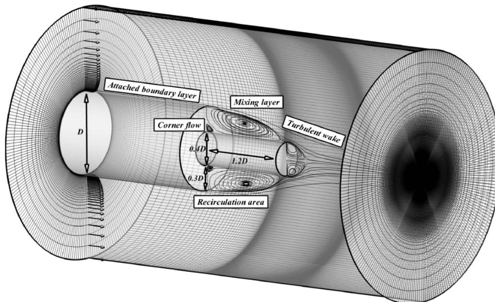
FIG. 1. Sketch of the geometry exhibiting the mesh, velocity vectors upstream from the separated area, characteristic dimensions, and the mean organization of the flow.
