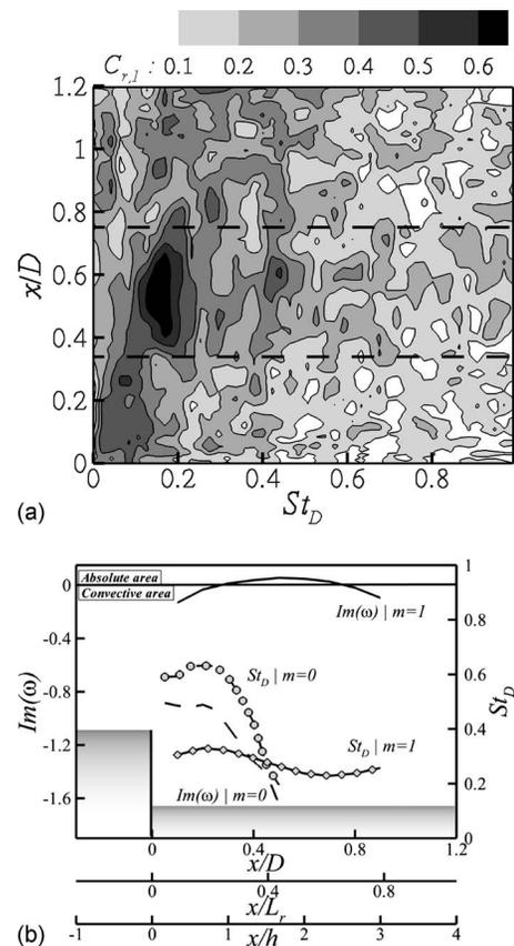
FIG. 8. (a) Spectral sheet of the azimuthal pressure mode  $C_{r,1}$  for every streamwise location along the emergence in function of nondimensional frequencies; (–) spatial limits of the absolute area for  $m=1$ . (b)  $m=0$  and  $m=1$  modes for the axisymmetric case; (–)  $\text{Im}(\omega)^{m=0}=f(x/D, x/L_r, x/h)$ , (–)  $\text{Im}(\omega)^{m=1}=f(x/D, x/L_r, x/h)$ , ( $\circ$ )  $St_D^{m=0}=f(x/D, x/L_r, x/h)$ , and ( $\diamond$ )  $St_D^{m=1}=f(x/D, x/L_r, x/h)$ .
