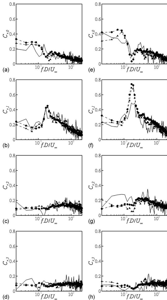
FIG. 7. [(a)–(d)] Spectra of the first four azimuthal pressure modes  $C_{r,0}$ ,  $C_{r,1}$ ,  $C_{r,2}$ , and  $C_{r,3}$  for the streamwise location  $x/D=1.15$ . ( $\blacktriangle$ ) Ref. 6, ( $\bullet$ ) Ref. 17, and (–) present calculation. [(e)–(h)] Spectra of the first four azimuthal pressure modes  $C_{r,0}$ ,  $C_{r,1}$ ,  $C_{r,2}$ , and  $C_{r,3}$  for the streamwise location  $x/D=0.72$ . ( $\blacktriangle$ ) Ref. 6, ( $\bullet$ ) Ref. 17, and (–) present calculation.
