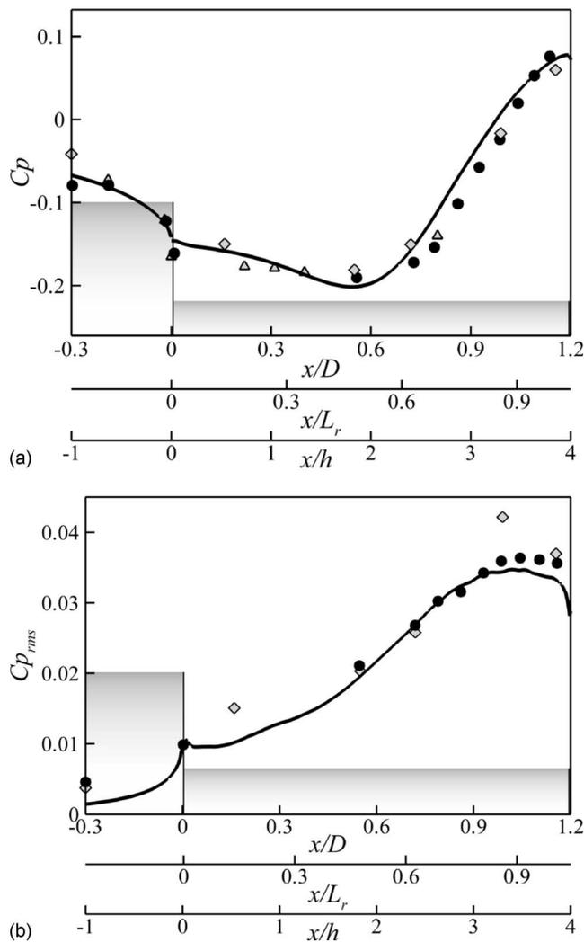
FIG. 3. (a) Streamwise distribution of the pressure coefficient. ( $\diamond$ ) Ref. 6 (kulites), ( $\triangle$ ) Ref. 6 (steady taps), ( $\bullet$ ) Ref. 17, and (—) present case. (b) Streamwise distribution of the coefficient of rms pressure fluctuation. ( $\diamond$ ) Ref. 6 (kulites), ( $\bullet$ ) Ref. 17, and (—) present case.
