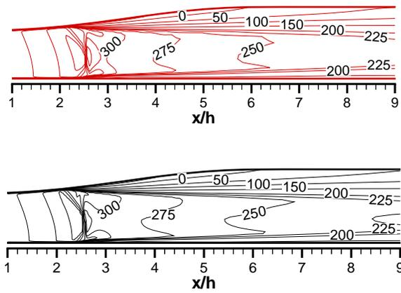
**Fig. 6**  $\bar{U}$  contours (m/s), computation. Top : (136x99) points, bottom : (136x111) points
