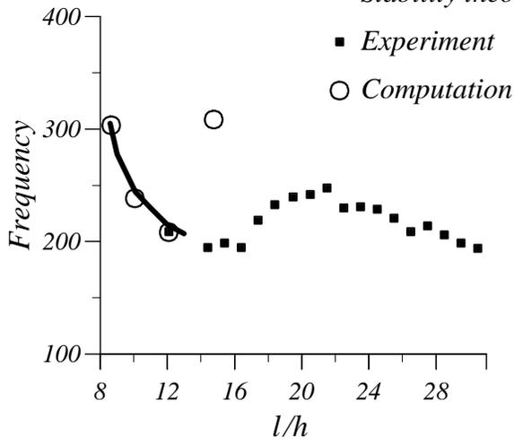
Fig. 11 Frequency versus diffuser length.
