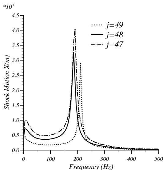
Fig. 10  $y$ -dependence of shock motion spectrum.
