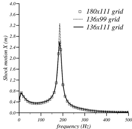
Fig. 9 Robustness of shock motion spectrum.
