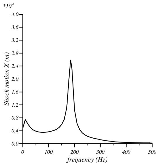
Fig. 8 Shock motion spectrum,  $l/h = 13$ .
