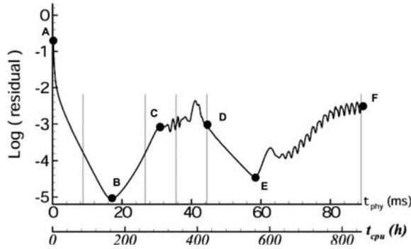
**Fig. 11** Residual time evolution and CPU time on a 2.4 GHz Pentium processor,  $L_z = 0.8$ ,  $\theta = 32^\circ$ .
