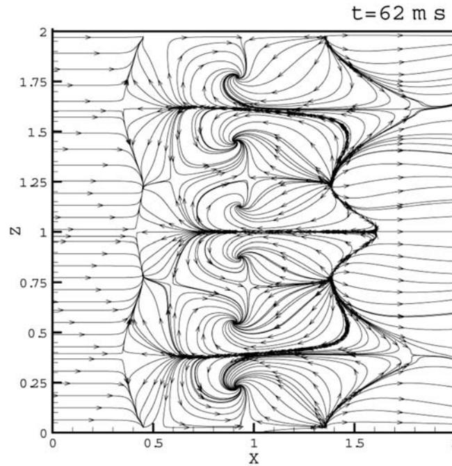
Fig. 15 Surface streamlines on the plate at  $t = 62 \text{ ms}$ ,  $\theta = 32^\circ$ ,  $L_z = 2$
