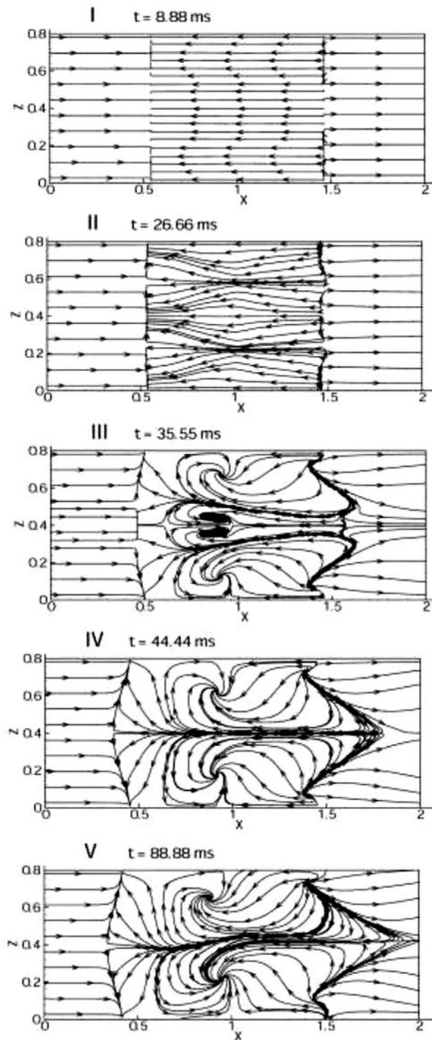
**Fig. 12** Surface streamlines on the plate at different moments,  $L_z = 0.8$ ,  $\theta = 32^\circ$
