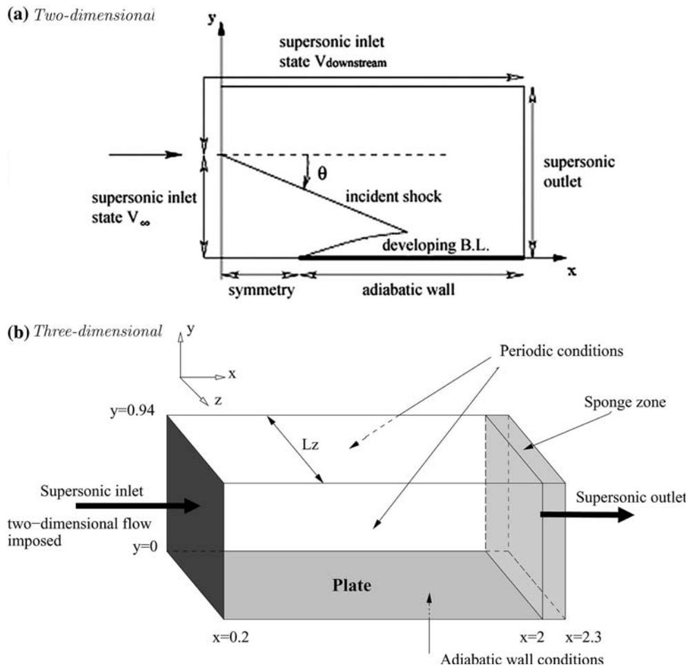
**Fig. 2** Computational domain and boundary conditions. (a) Two-dimensional (2D), (b) Three-dimensional (3D)
