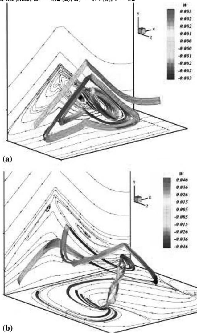
Fig. 6 3-Dimensional view inside the bulb,  $L_z = 0.2$  (a),  $L_z = 0.4$  (b),  $\theta = 32^\circ$
