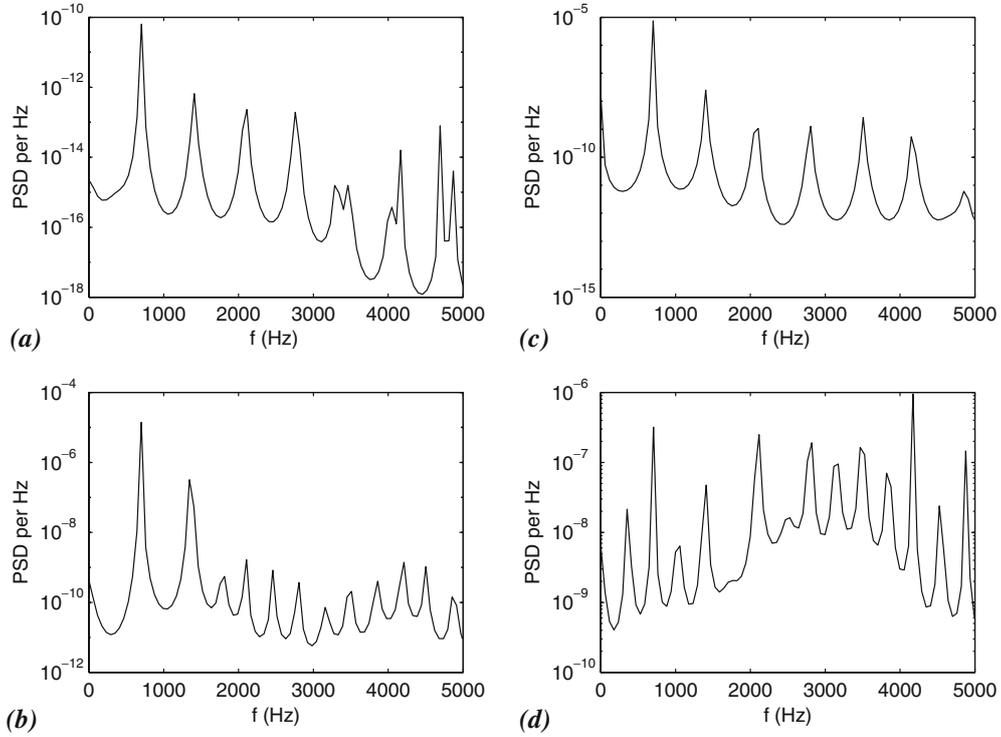
**Fig. 10** Pressure spectra density for different points in the flow. **a**  $(x_0, y_0, z_0) = (0.8053, 0.6, 0.4)$ , **b**  $(0.8053, 0.28, 0.4)$ , **c**  $(0.8053, 0.18, 0.4)$  and **d**  $(0.8053, 0.042, 0.4)$  for  $\theta = 32.5^\circ$  and  $L_z = 0.8$
