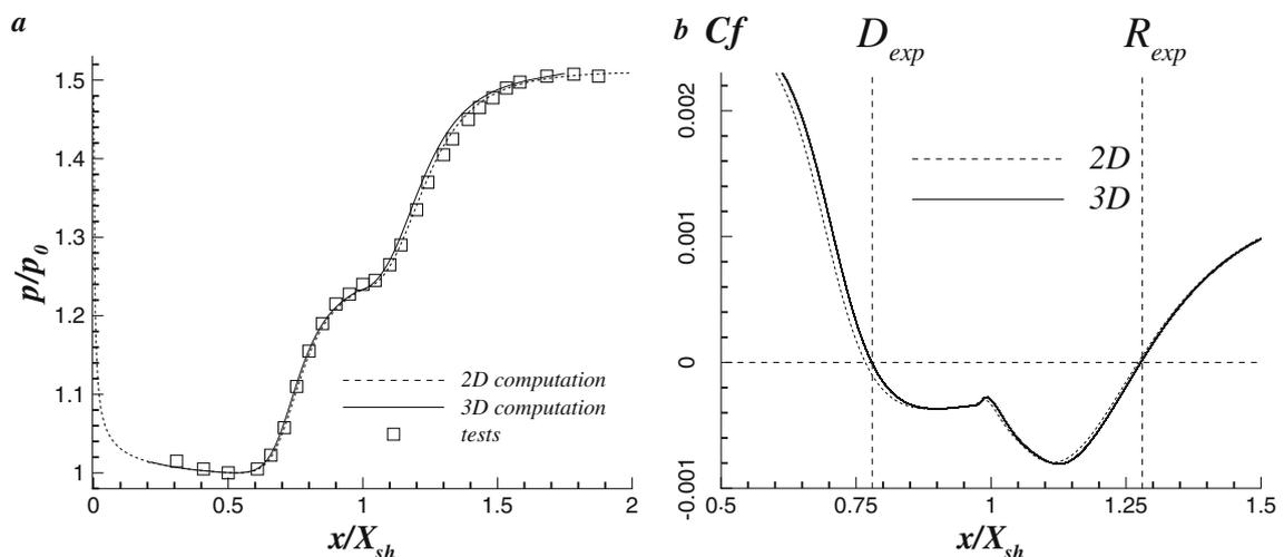
Fig. 3 Shock/boundary layer interaction. Pressure (a) and skin-friction distribution (b) along the plate
