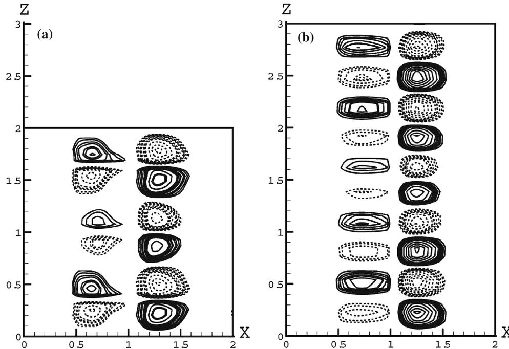
Fig. 16  $z$ -Component of the friction coefficient on the plate,  $\theta = 32^\circ$ ,  $L_z = 2$  (a),  $L_z = 3$  (b)
