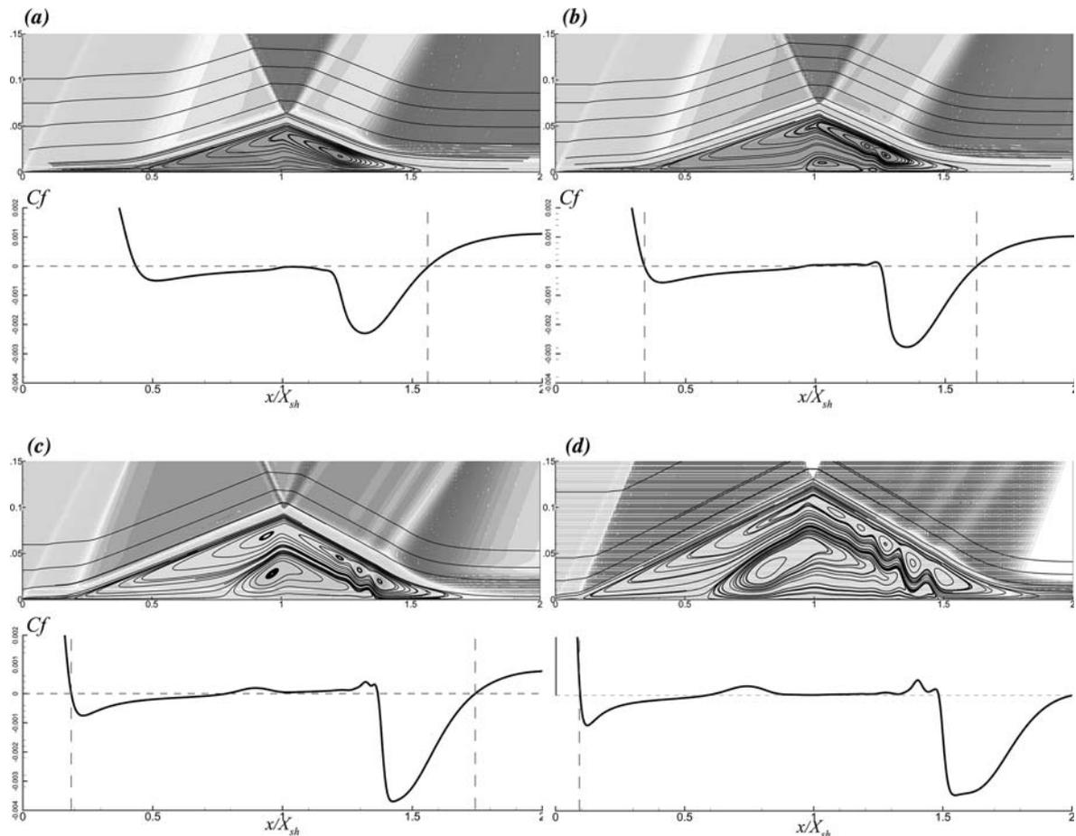
**Fig. 4** Isochors and streamlines, skin-friction coefficient for  $\theta = 32.5^\circ$  (a),  $33^\circ$  (b),  $\theta = 34^\circ$  (c) and  $35^\circ$  (d) vertical to longitudinal ratio is 3.5
