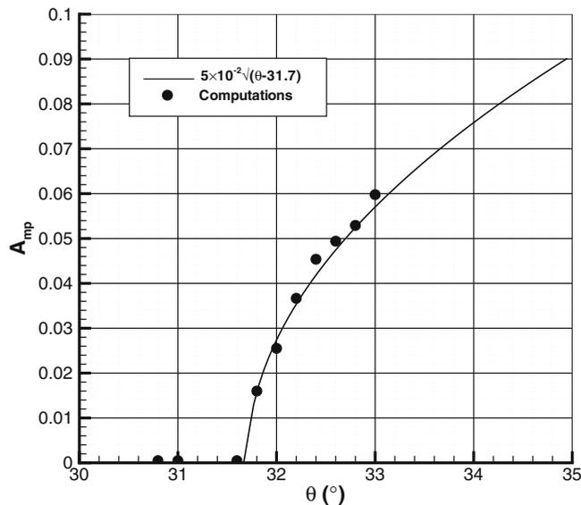
**Fig. 8** The amplitude of the oscillations of  $w$  as a function of  $\theta$ . • Numerical simulations, line :  $A_{mp} \sim \sqrt{\theta - 31.7}$  at  $(x_0, y_0, z_0) = (1, 5 \times 10^{-2}, 0.4)$ ,  $L_z = 0.8$
