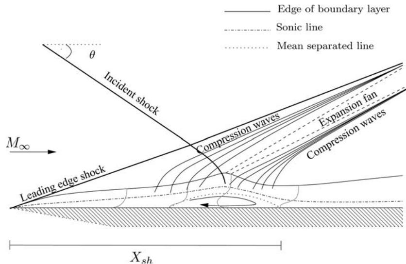
Fig. 1 Schematic representation of the shock wave/boundary layer interaction
