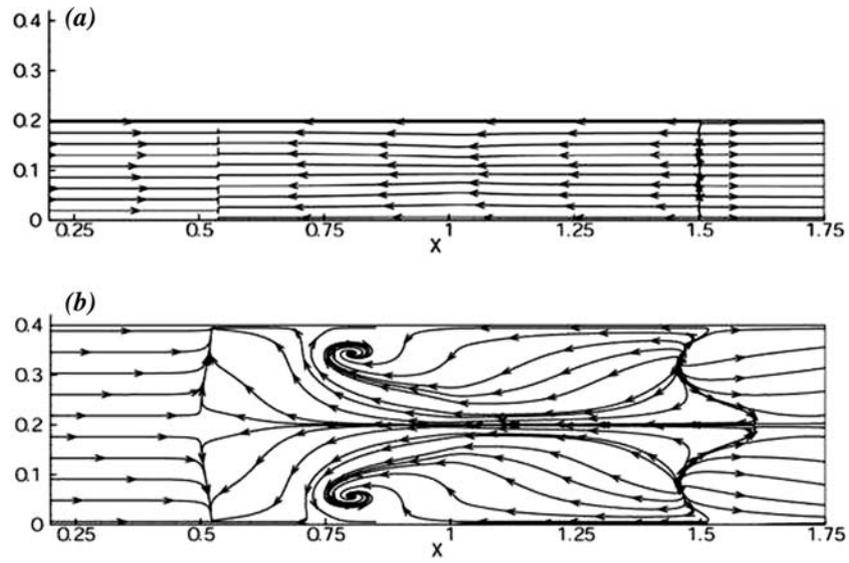
Fig. 5 Surface streamlines on the plate,  $L_z = 0.2$  (a),  $L_z = 0.4$  (b),  $\theta = 32^\circ$
