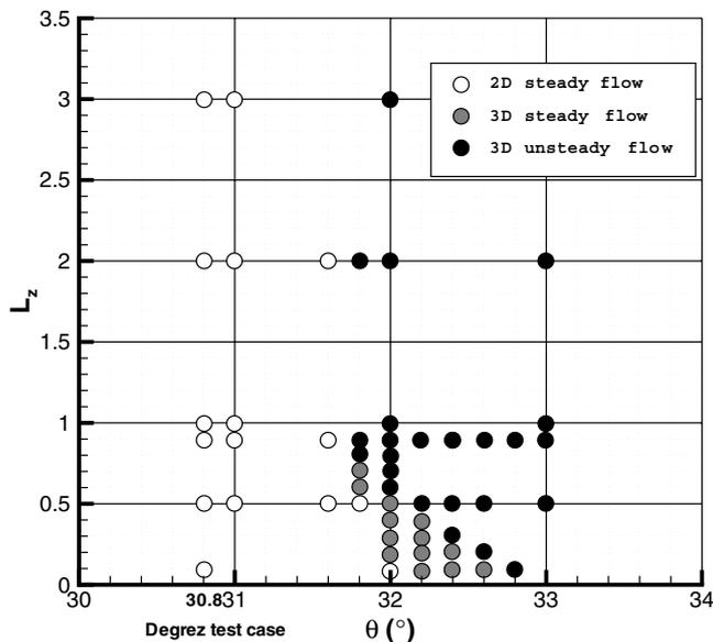
Fig. 17 Flow organization according to the incident shock angle and the transverse size of the computation domain
